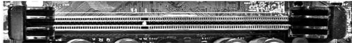
Slot 1 / SC242 - Intel Celeron SEPP, Pentium II, Pentium III - 242 pins
