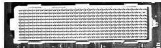
Apple G3/G4/G5 Processor card socket - 300 pins
